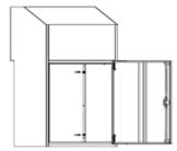
**Please note:** depending on the depth of your fence you may need to put spacer between the back of your fence and the parcel box to ensure the front of the parcel box is flush with the front of the fence.
