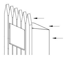
3. Fix it to the fence with the screws provided using the 4 pre-drilled holes in the front of the back box. (for hardwood fences, it is easier to pre-drill the screw holes). This step will be easier with two people.
